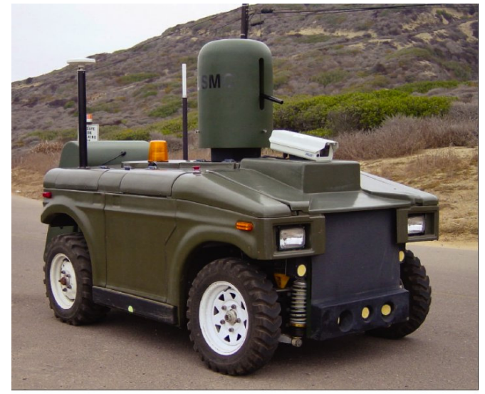
MDARS-E Prototype Platform with Gunpod
