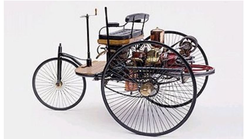
First Car: 1886 Benz Patent Motor Car (single-cylinder four-stroke engine)
