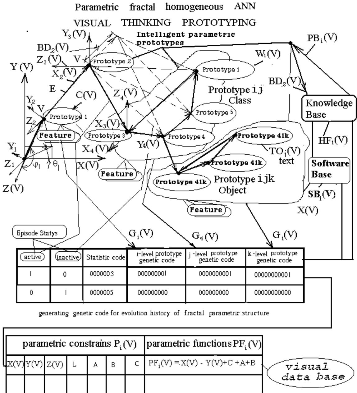
Fig. 1. A schematic representation of IPPMS control strategies. The model generates the fractal tree using a family of homogeneous matrices. A key step in the structural recovery is the formation of cellular encoding with genetic code of each node of fractal network.
