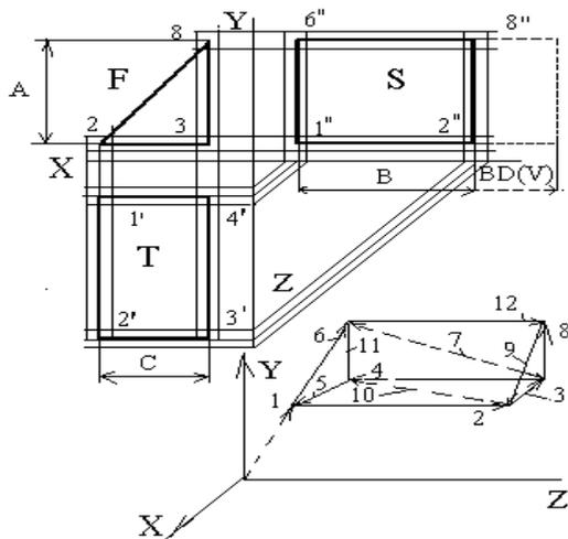
Fig. 4. The scheme for 3D object reconstruction from views using IPPMS.
